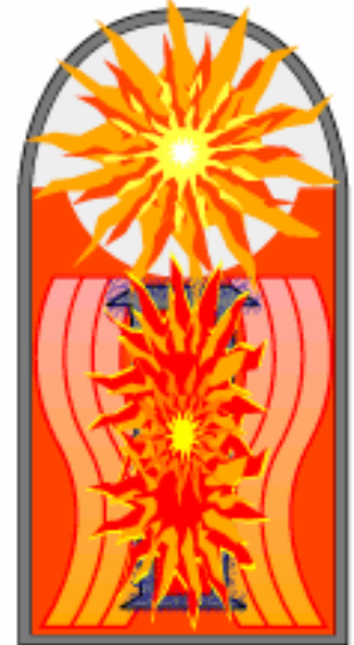
5. Compressed and heated, lithium-6 deuteride fuel begins fusion reaction, neutron flux causes tamper to fission. A fireball is starting to form...
